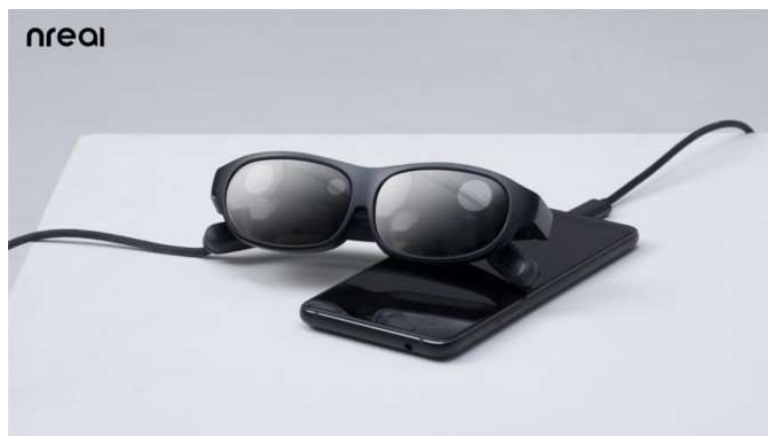
Figure 1: The Nreal Light AR glasses tethered to a high-end Android smartphone.
